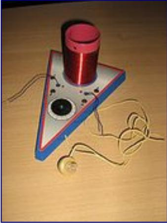
Modern crystal radio with [piezoelectric earphone](#)
