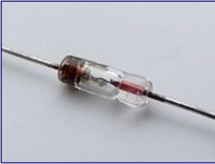
Germanium diode used in modern crystal radios (about 3 mm long)
