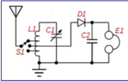
Direct-coupled circuit with impedance matching[46]
