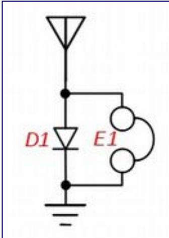
The earliest crystal receiver circuit did not have a [tuned circuit](#)
