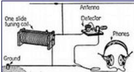
Pictorial diagram from 1922 showing the circuit of a crystal radio. This common circuit did not use a tuning [capacitor](#), but used the capacitance of the antenna to form the [tuned circuit](#) with the coil. The detector might have been a piece of galena with a whisker wire in contact with it on a part of the crystal, making a diode contact
